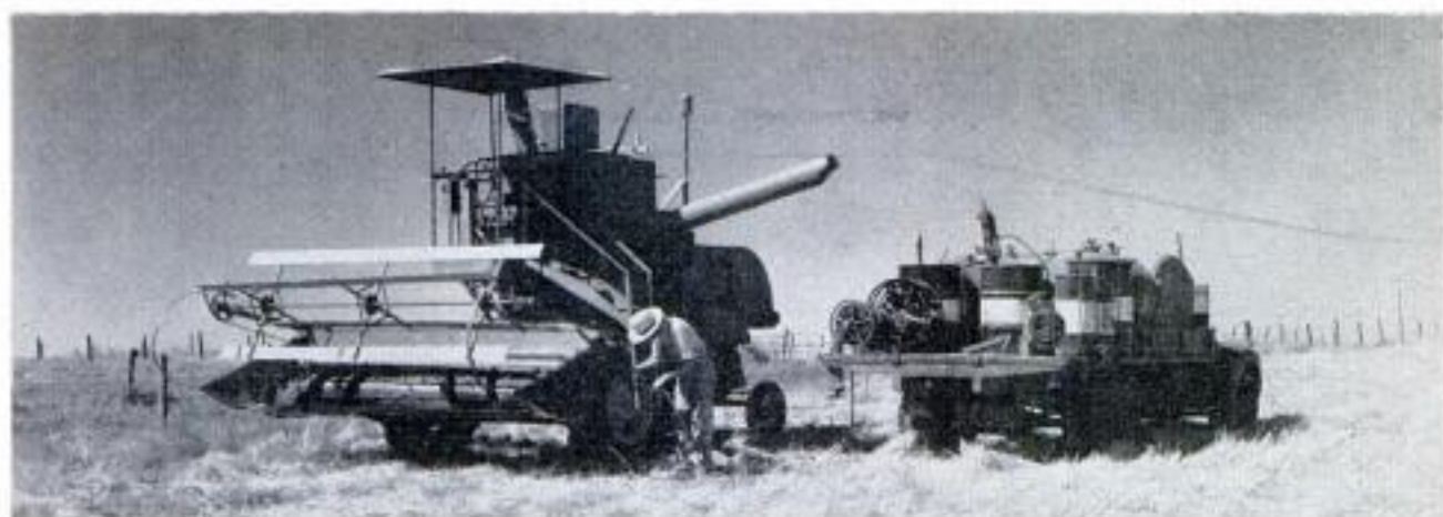
Superservice rolls into the field. With the equipment packed on truck, this combine can be serviced in 10 minutes
